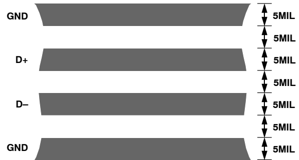
Figure 21. Typical Arrangement of Signal Tracks
